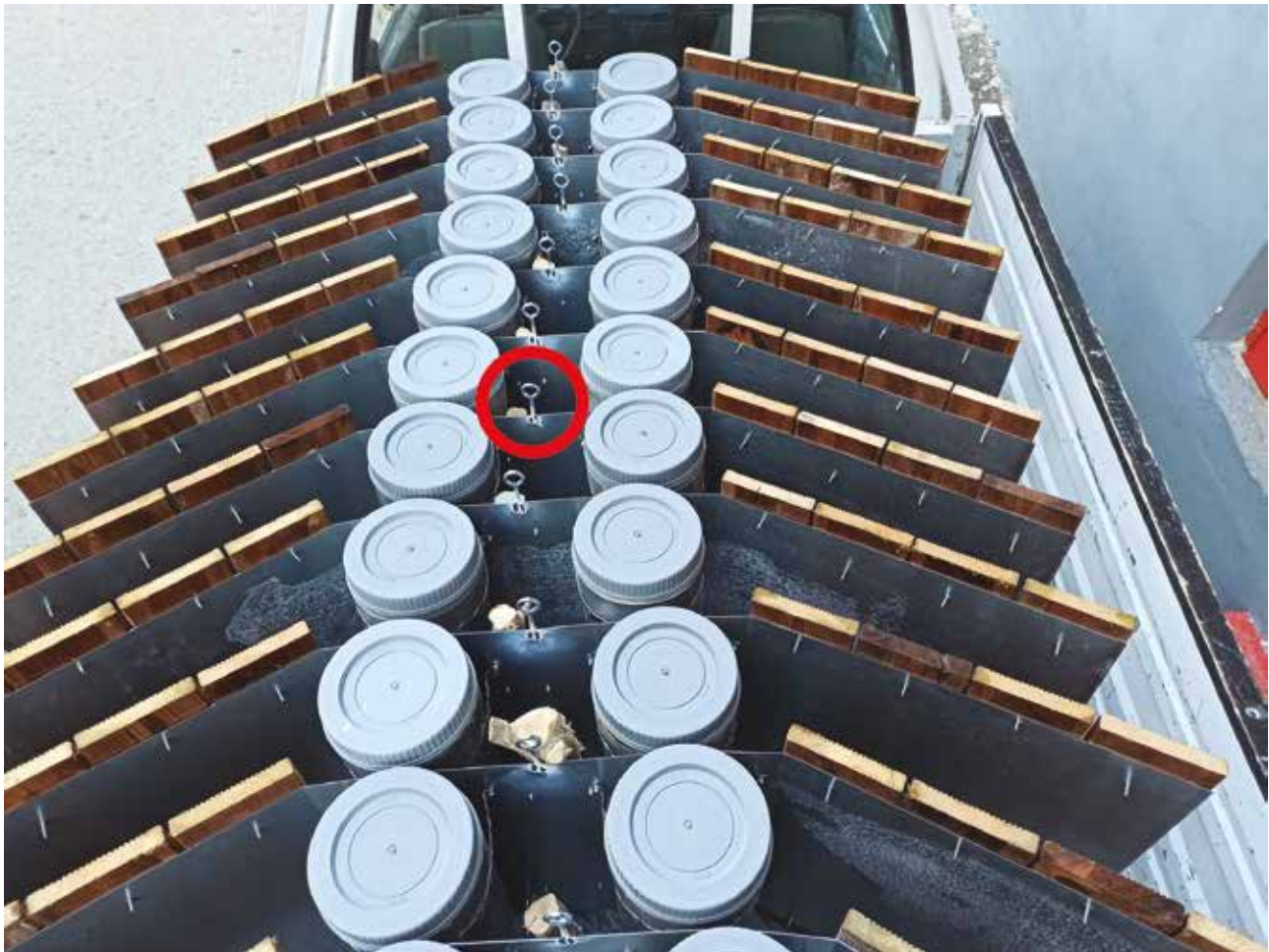
Figure 12: Detail (eye bolt) of the model escape devices constructed in the framework of LIFE Bonelli eastMed. ©UoC-NHMC Archive.
